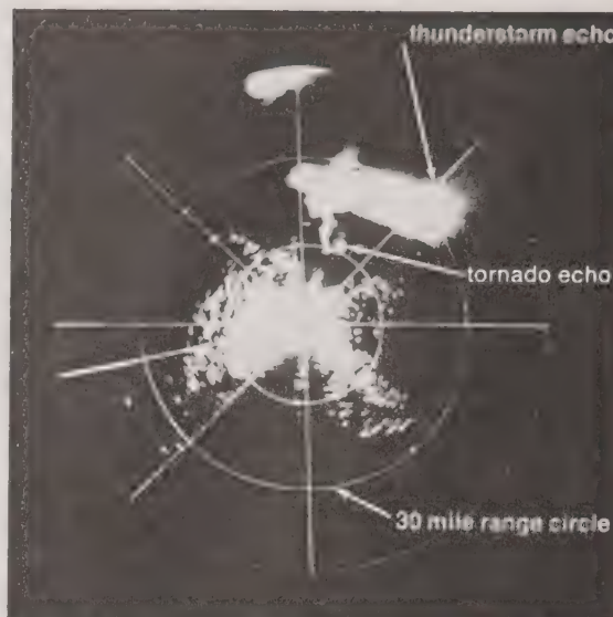
Figure 45: Hook echo of a tornado in Champaign, Ill., photographed on a radar scope on April 9, 1953. This was the first occasion on which the hook echo, an important clue in the tornado warning system, was recognized and photographed.
